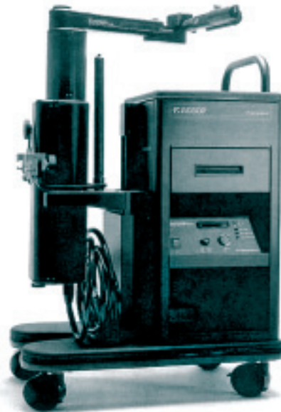
Fig.1 AESOP™ (Automated Endoscopic System for Optimal Positioning) voice-controlled robotic arm.
