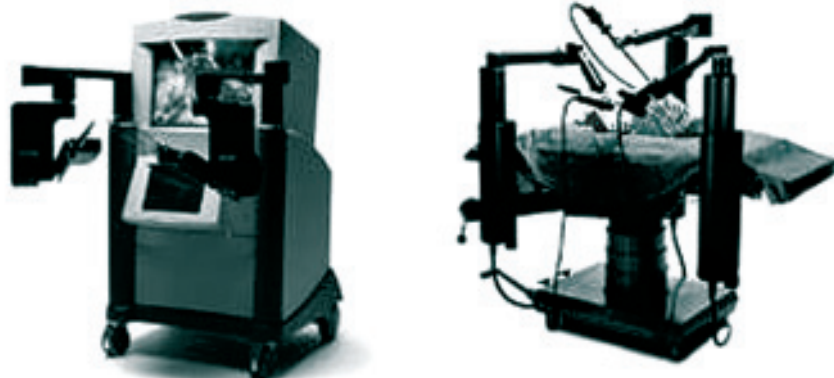
Fig.2 The ZEUS™ robotic microsurgical system. Surgeon’s console and surgical cart with the three robotic arms attached to the operating table.
