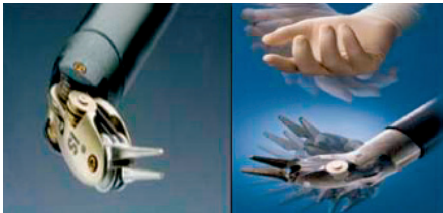
Fig.4 Endowrist instrument which translates surgeon's hand and wrist movements into precise laparoscopic instrument movements with 7 degrees of freedom of motion inside the abdomen.
